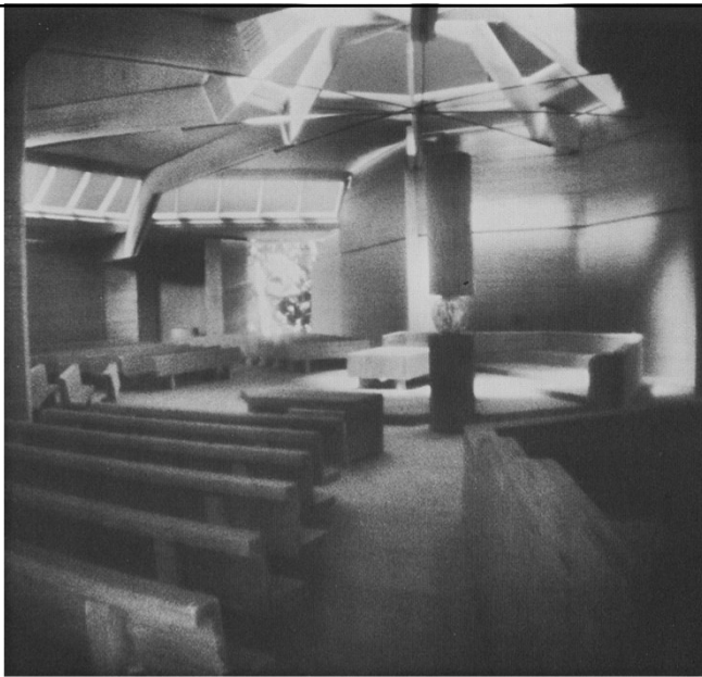
interior model: Gerhard Haisch: Parish centre St. Stephan, Munich 1975, 1977. Scale 1:50. Base in plywood, construction of building in balsa wood.
