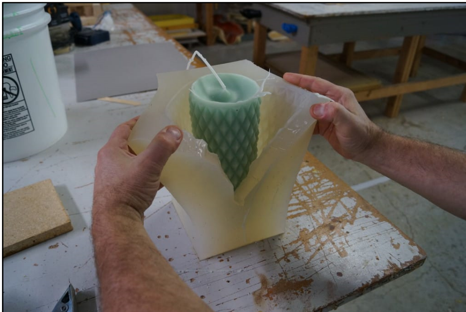
Silicon rubber candle mould. Making of: https://www.polytek.com/tutorial/tutorial-how-make-silicone-rubber-candle-mold
