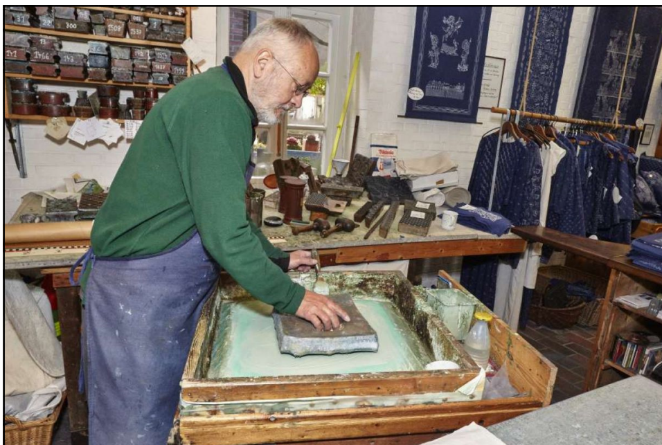
Jever, blue print workshop. The blue printer presses the mould into the paste.
